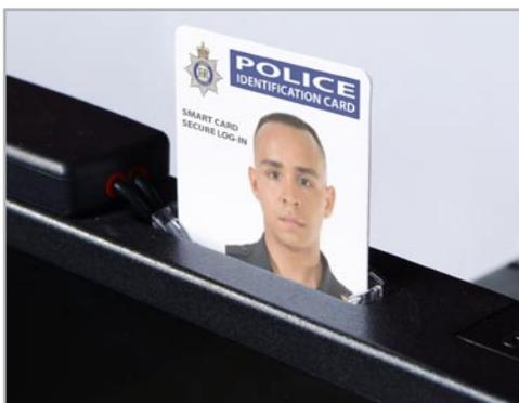
The built in SMART CARD reader enables the MDT to only be used by authorised personnel. It also means that if the card is removed (during an on foot pursuit) the system can be locked, securing the sensitive access to data.
