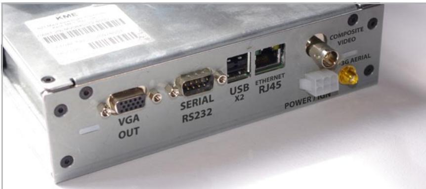
Standard PC connector interfaces are brought out on the rear of the DIN housing. RS232 serial 9 way 'D' (can be used to interface with a range of equipment e.g tracker). USB, to interface with any peripherals like a keyboard. 3G SMA aerial port, only needed if the signal needs to be boosted in a particularly bad signal area. There is also a removable cover on the side of the DIN which provides access to the SSD hard drive and SIM CARD.
